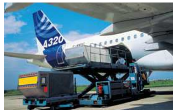
The A320 offers a choice between bulk or containerised baggage and cargo to maximise upload during short turns.
